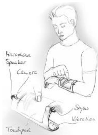
Figure 1: The armband prototype includes a large touch display, a camera, and an optional stylus.
